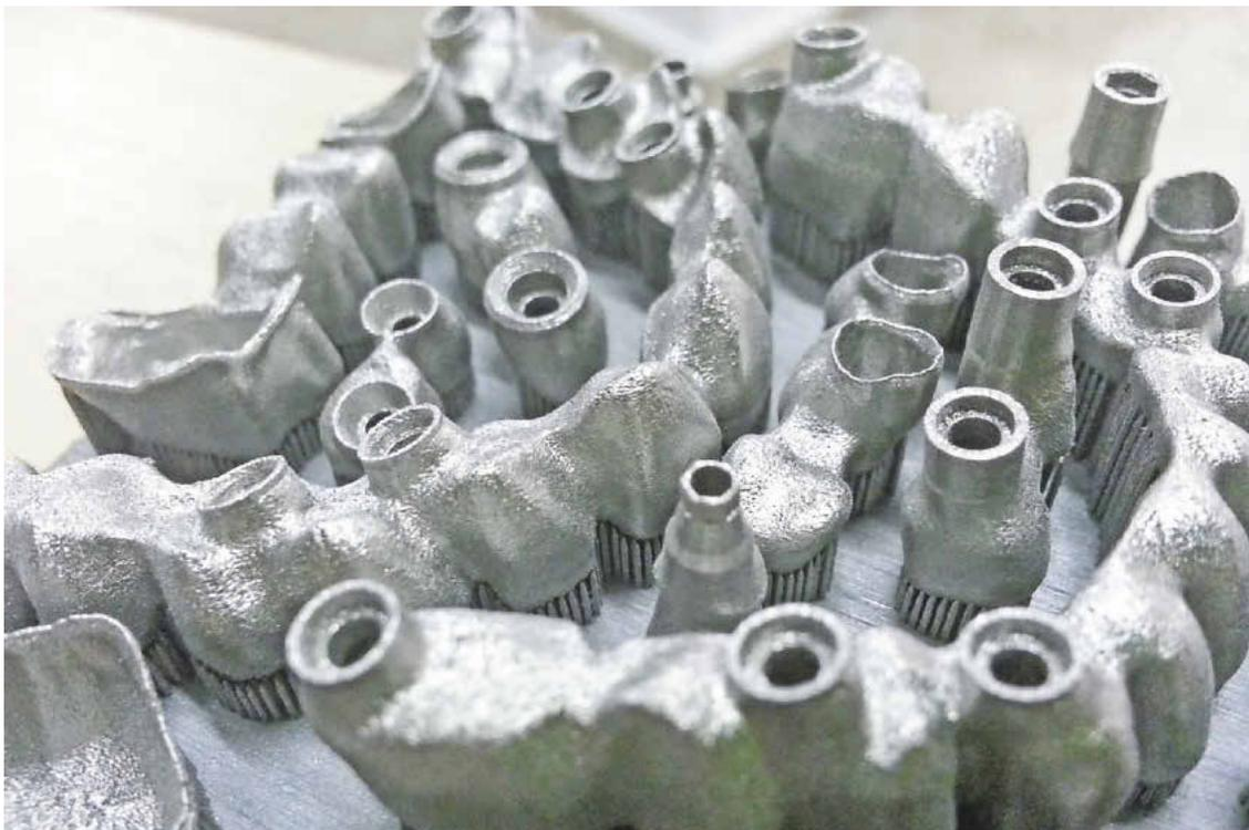
Metal laser melting technology is used to make abutments, crowns, and bridges in a single step—on a shared base plate with supporting structures.
